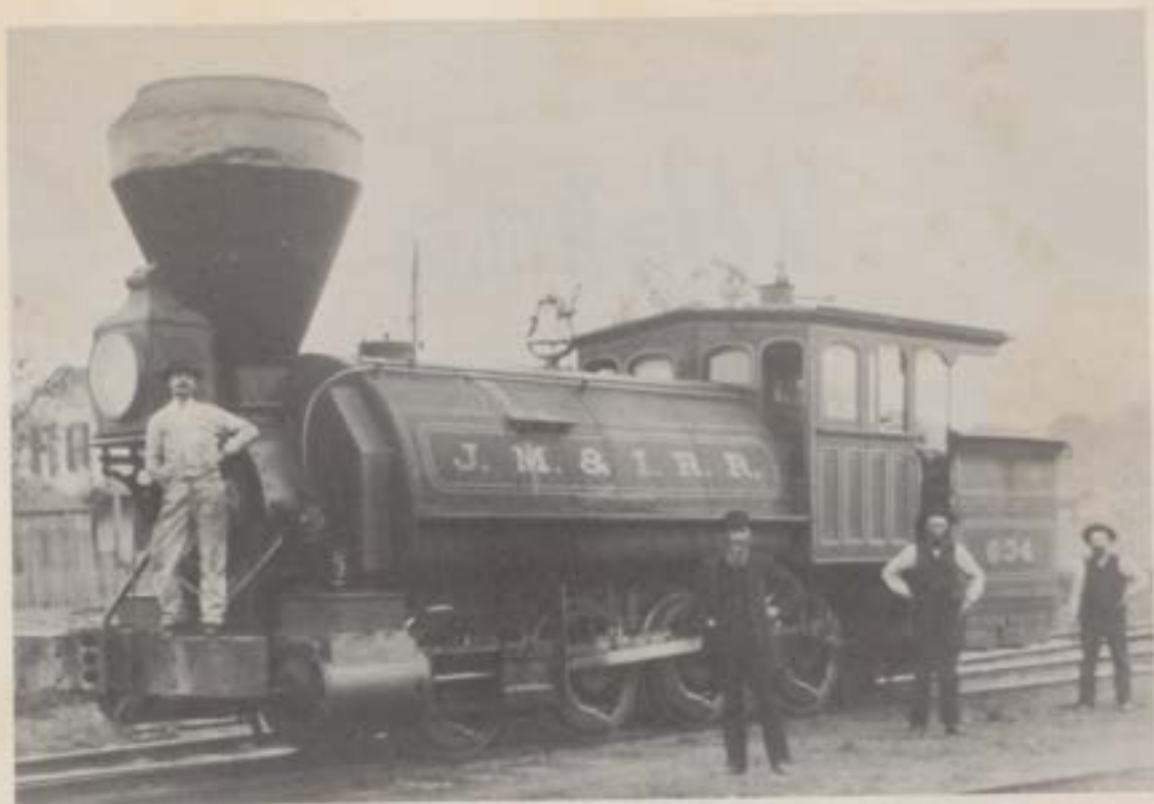
Locomotive built by the Jeffersonville, Madison, and Indianapolis Railroad Company to work on the inclined plane at Madison, Indiana.
