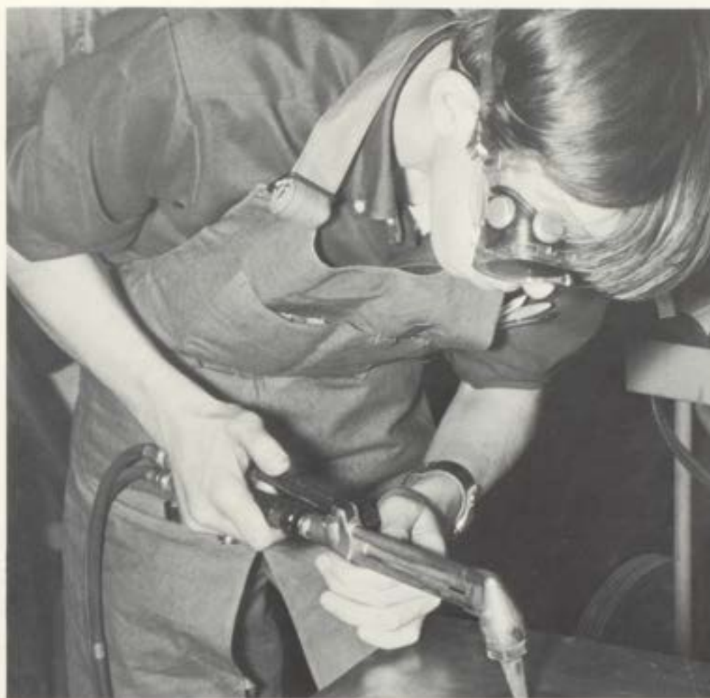
Learning the proper technique to use the acetylene cutting torch is one of the skills obtained in industrial arts. Gary Kelly is cutting a hole in metal to make a plate for a switch.
