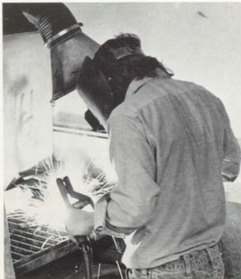
Sparks fly as Jim O'Neal spot welds two pieces of sheet metal.
